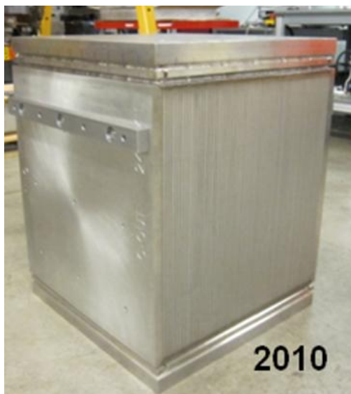
Figure 11. Commercial microchannel manufacturing techniques validated for FT reactor architecture
